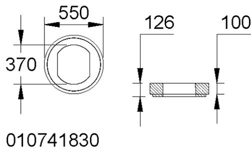
**MEACRET LINE 200 ADAPTATEUR POUR RACCORDEMENT DES AVALOIRS**
